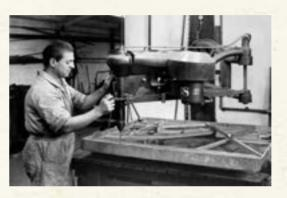
Beale set out in 1893 to manufacture every element of his pianos. Seen here is the precision drilling of the iron frame to ensure correct positioning and angle of all the tuning pins.
